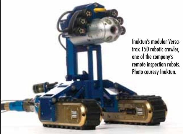
Inuktun's modular Versatrax 150 robotic crawler, one of the company's remote inspection robots. Photo courtesy Inuktun.
