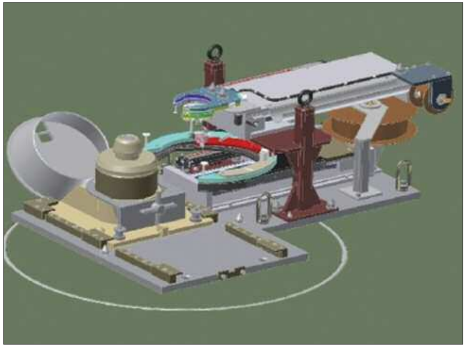
A 3-D computer rendering of the remote orbital welding station (Graphic: DSRL/NDA)
