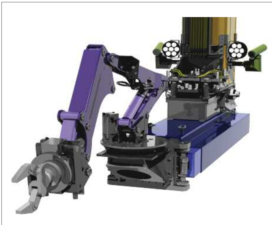
Computer image of the reactor dismantling manipulator, also known as "Reactorsaurus" (Graphic: DSRL/NDA)
